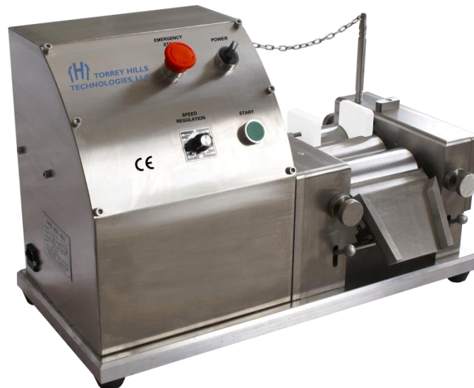
Figure 4. Torrey Hills T65 three roll mill used for CNT dispersion into a polymer matrix
