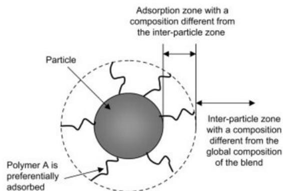
**Figure 1.** Partially miscible polymer blend with a polymer interacting with the filler [13]
