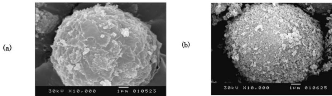
**Figure 2.** SEM images of coated particles. (a) is produced by a hybridizer and (b) is produced by a mill with high compression and shearing ability [1]
