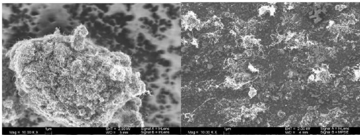
*Figure 3. Carbon nanotube agglomeration on the left and agglomeration reduction on the right [8]*
