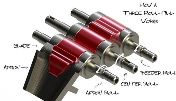
*Figure 4. How a three roll mill works.*
